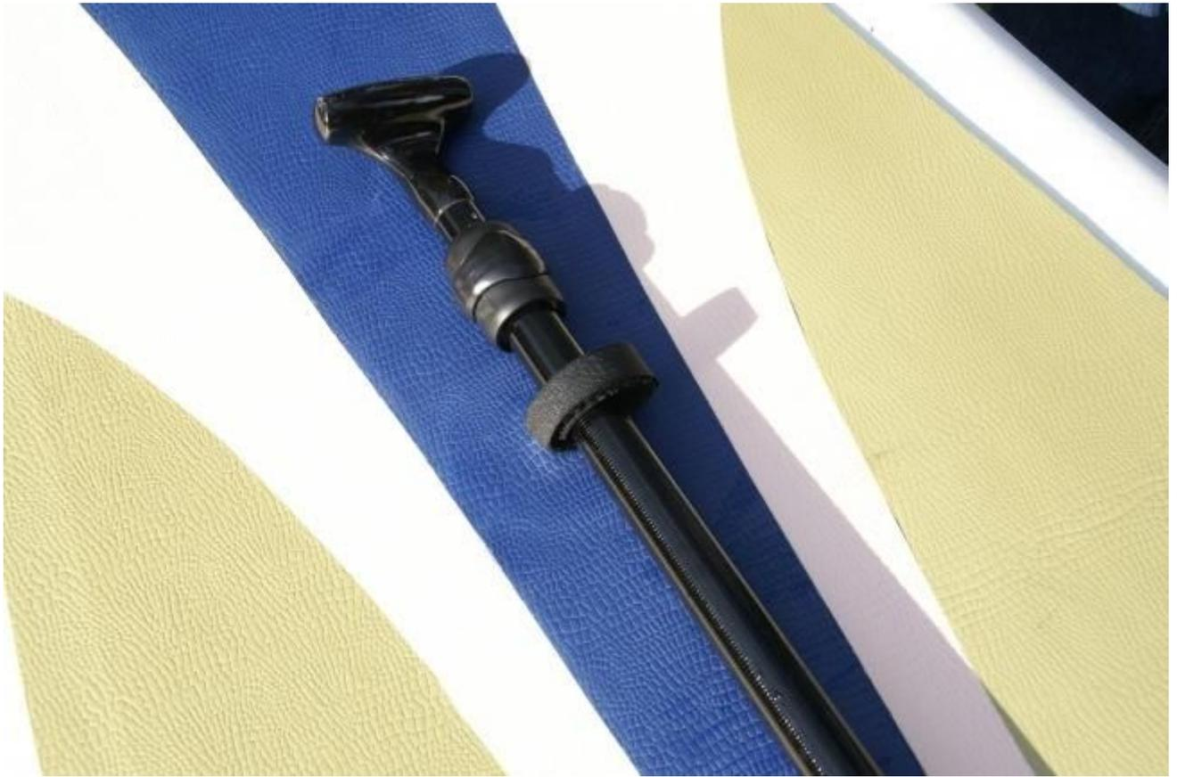
**Step 6:** Attach the paddle onto the top of the board using the 2 velcro straps (for 2011 and older boards)
